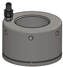
HNST Hydraulic Nuts are used in direct replacement of the existing conventional nut. They allow accurate loading of the bolt, and the load is then permanently retained by means of a shim inserted between the nut body and piston equal to the bolt elongation (plus joint compression).
